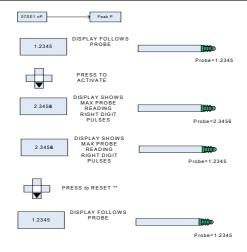
\*\* THE SI1000 WILL REMAIN IN PEAK P MODE UNTIL THE TIME SET IN MENU 08 HAS COMPLETED. PEAK-N AND DIFF MODES OPERATE IN THE SAME WAY
