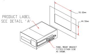
Working from behind the panel, with the box fully located, fit the side brackets to the studs and slide them forward toward the panel until they lock into place.
